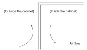
When air flows along the outer wall of the cabinet, effective heat exchange will be possible, because the temperature slope inside and outside the cabinet will be steeper.
