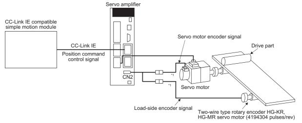
\*1 Use a two-wire type encoder cable. A four-wire type linear encoder cable cannot be used.
