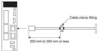
When using a data line filter
