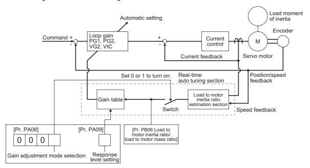
When a servo motor is accelerated/decelerated, the load to motor inertia ratio estimation section always estimates the load to motor inertia ratio from the current and speed of the servo motor. The results of estimation are written to [Pr. PB06 Load to motor inertia ratio/load to motor mass ratio]. These results can be confirmed on the status display screen of the MR Configurator2.
