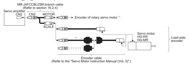
\*1 Use a two-wire type encoder cable. A four-wire type linear encoder cable cannot be used.
