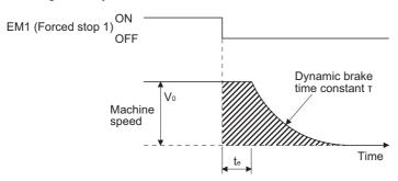
$$L_{\text{max}} = \frac{V_0}{60} \cdot \left\{ t_e + \tau \left( 1 + \frac{J_L}{J_M} \right) \right\} \dots (15.1)$$
