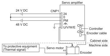
\*1 Please use a thermal sensor, etc. for thermal protection of the servo motor.
