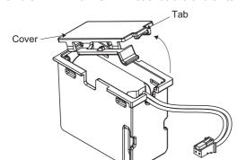
2. Replace the battery with a new MR-BAT6V1 battery.
