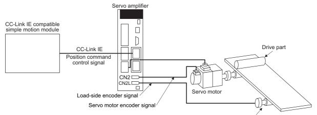
A/B/Z-phase differential output, two-wire type, or four-wire type rotary encoder HG-KR, HG-MR servo motor (4194304 pulses/rev) or synchronous encoder Q171ENC-W8 (4194304 pulses/rev)
