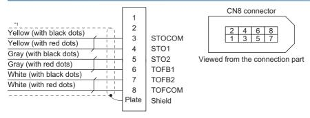
\*1 Do not use the two core wires with orange insulator (with red or black dots).
