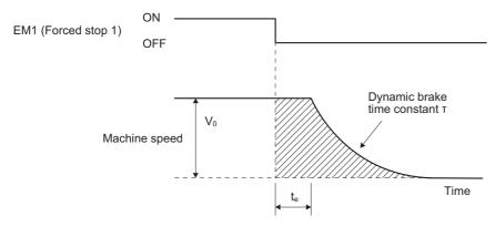
$$L_{\text{max}} = \frac{V_0}{60} \cdot \left\{ t_e + \tau \left( 1 + \frac{J_L}{J_M} \right) \right\} \quad \dots (10.2)$$
