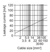
"Ig1" of 100 V class servo amplifiers is 1/2 of 200 V class servo amplifiers.
