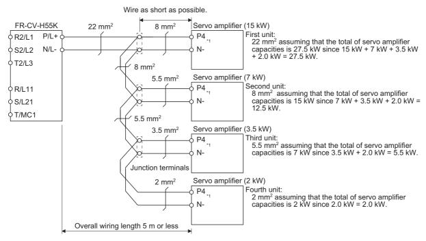
\*1 When using the servo amplifier of 7 kW or less, make sure to disconnect the wiring of built-in regenerative resistor (5 kW or less: P+ and D, 7 kW: P+ and C).
