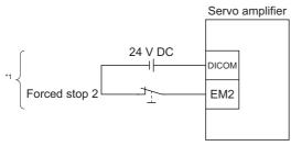
\*1 This diagram shows sink I/O interface. For source I/O interface, refer to the following.
