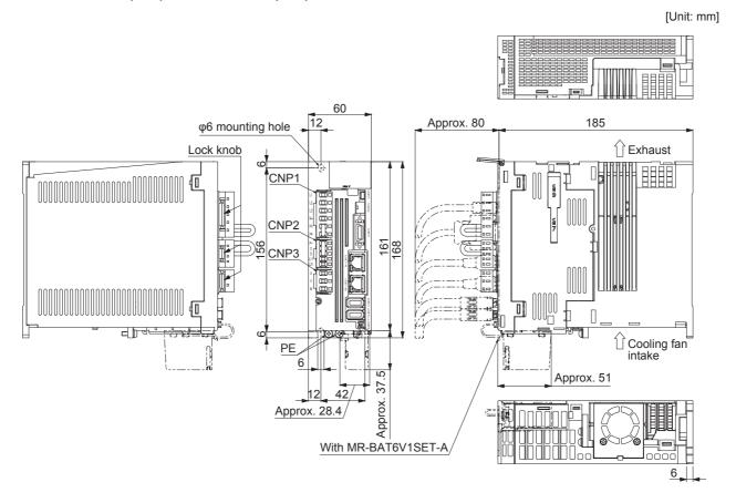
Terminal CNP1 L1 L2 L3 N-РЗ P4 CNP2 P+ С D L11 L21 CNP3 U ٧ W PE Screw size: M4 **(**  $\oplus$ Tightening torque: 1.2 [N•m]
