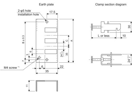
1 Screw hole for grounding. Connect it to the grounding plate of the cabinet.
