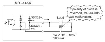
\*1 If the voltage drop (maximum of 2.6 V) interferes with the relay operation, apply high voltage (maximum of 26.4 V) from external source.
