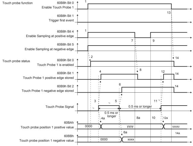
\*1 Turn on and off Touch Probe Signal so that both the on time and off time are 0.5 ms or longer.
