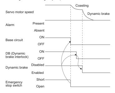
· Timing chart when both of the main and control circuit power are off
