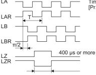
Time cycle (T) is determined by the settings of [Pr. PA15] and [Pr. PC03].
