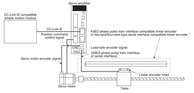
\*1 Applicable for the absolute position detection system when an absolute position linear encoder is used. In that case, a battery is not required.
