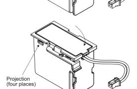
**3.** Press the cover until it is fixed with the projection of the locking part to close the cover.
