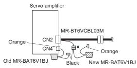
**3.** Remove the orange connector of the old MR-BAT6V1BJ. When the control circuit power supply is on, performing 3) without [AL. 9F.1 Low battery] triggers [AL. 9F.1].
