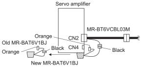
**5.** Mount the orange connector of the new MR-BAT6V1BJ. When the control circuit power supply is on, [AL. 9F.1] is canceled.
