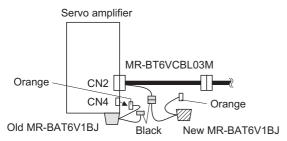
**4.** Remove the old MR-BAT6V1BJ from servo amplifier and mount the new MR-BAT6V1BJ. When the control circuit power supply is on, [AL. 9F.1] occurs after 3).
