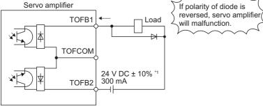
\*1 If the voltage drop (maximum of 5.2 V) interferes with the relay operation, apply high voltage (maximum of 26.4 V) from external source.
