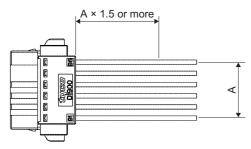
• Be sure that wires are not pulled excessively when the connector is inserted.
