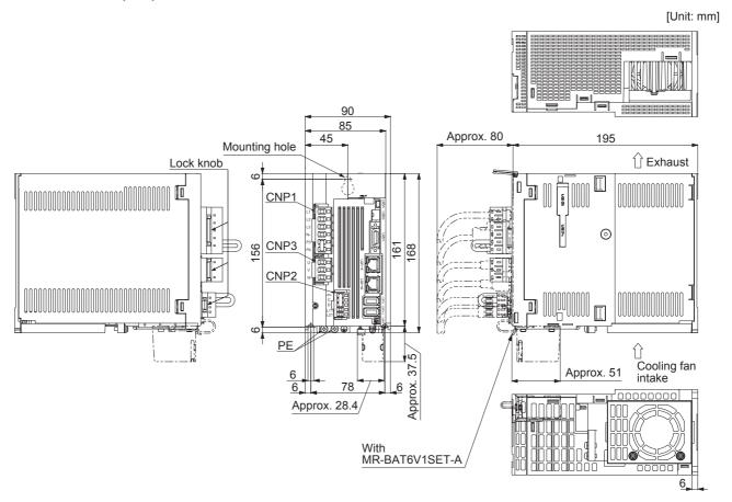
Mounting screw Terminal Screw size: M5 CNP1 Tightening torque: 3.24 [N•m] L1 L2 L3 Approx. 90 9 N-P3 P4 CNP3 V W Approx. 168  $156 \pm 0.5$ CNP2 φ13 hole 3-M5 screw С Mounting hole dimension D L11 Approx. 6 L21 PΕ Approx. 6 Approx. 6 Screw size: M4  $78 \pm 0.3$ **(1) (1)** Tightening torque: 1.2 [N•m] Mounting hole process drawing
