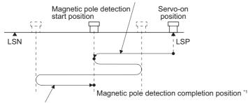
The linear servo motor reciprocates several times and returns to the magnetic pole detection start position to complete the magnetic pole detection and to go into the servo-lock status. At this time, there may be a gap, approximately a quarter of the pitch against magnetic pole, from the start position.
