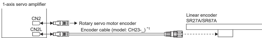
\*1 This optional cable is manufactured by Magnescale and should be prepared by the customer.
