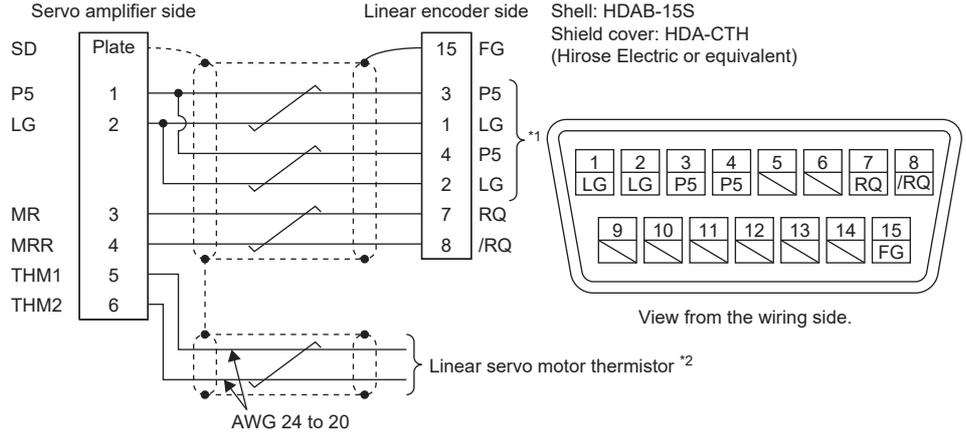
\*1 Encoder cables that meet the following specifications are recommended.
