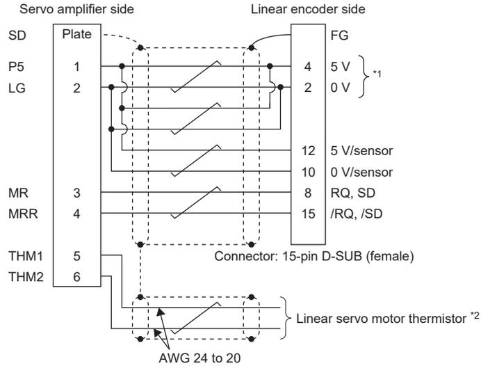
\*1 Encoder cables that meet the following specifications are recommended.
