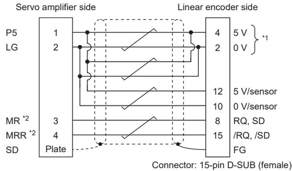
\*1 Encoder cables that meet the following specifications are recommended.
