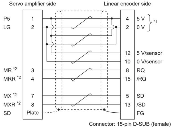
\*1 Encoder cables that meet the following specifications are recommended.
