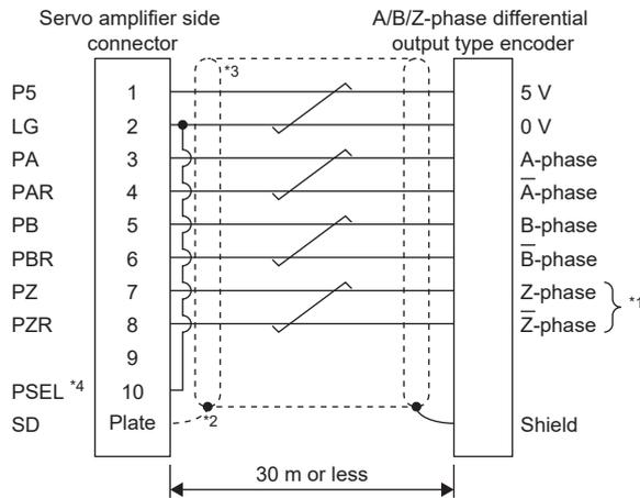
\*1 For the encoder without the Z-phase, set [Pr. PC45.2] (MR-J5-\_A\_-RJ) or [Pr. PC27.2] (MR-J5-\_G\_-RJ\_, MR-J5-\_B\_-RJ, or MR-J5D1\_) to "1".
