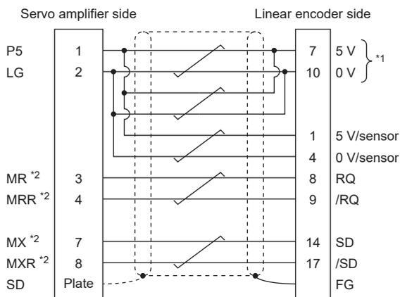
Connector: 17-pin coupling
