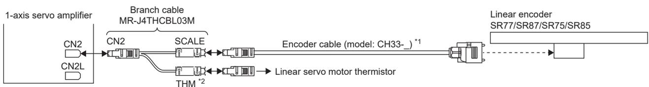
\*1 This optional cable is manufactured by Magnescale and should be prepared by the customer.
