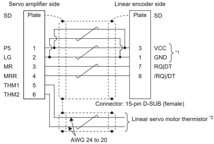
\*1 Encoder cables that meet the following specifications are recommended.
