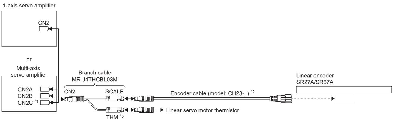
\*1 The connection to CN2C is for the MR-J5W3- and MR-J5D3- \_G\_. The MR-J5W2- and MR-J5D2- \_G\_ do not have CN2C.
