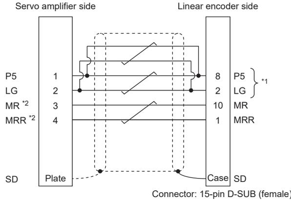
\*1 Encoder cables that meet the following specifications are recommended.
