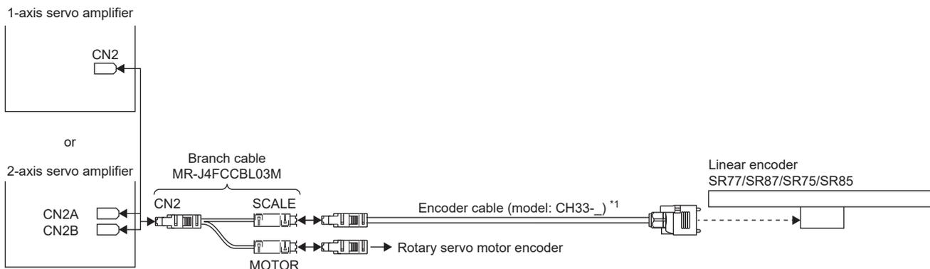
\*1 This optional cable is manufactured by Magnescale and should be prepared by the customer.
