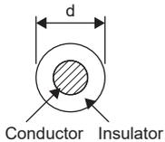
\*2 Standard OD. The maximum OD is about 10 % greater for dimensions without tolerances.
