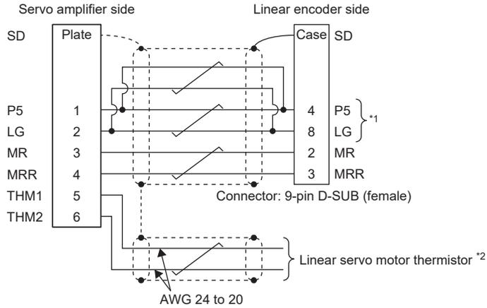
\*1 Encoder cables that meet the following specifications are recommended.
