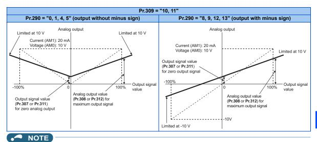
• When **Pr.307 = Pr.308** and **Pr.311 = Pr.312**, the output values from the terminals AM0 and AM1 will always be the values that are set in the parameters.
