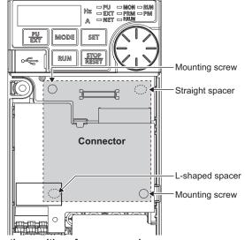
Insertion positions for screws and spacers
