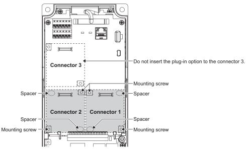
Insertion positions for screws and spacers
