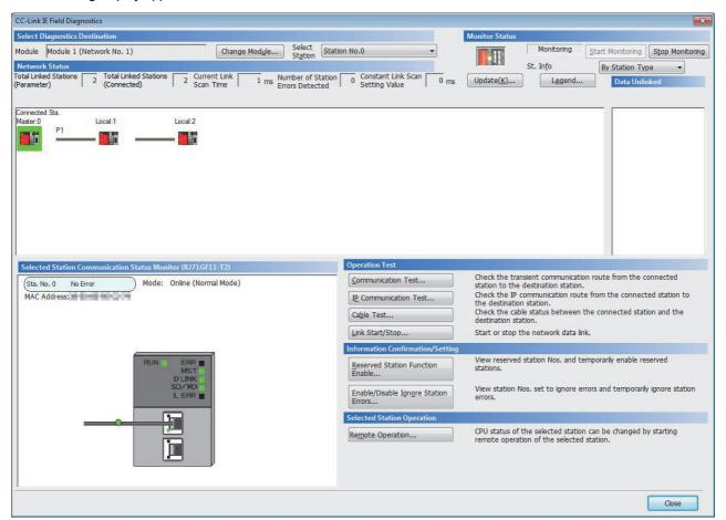
When an icon indicating an error is displayed in "Network Status" in "CC-Link IE Field Diagnostics", use the CC-Link IE Field Network diagnostics to identify the cause of the error and take actions. ( MELSEC iQ-R CC-Link IE Field Network User's Manual (Application))
