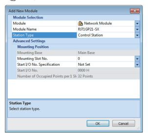
5. Click the [OK] button to add the module labels of the CC-Link IE Controller Network-equipped module.
