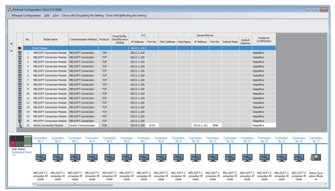
8. Write the set parameters to the CPU module. Then reset the CPU module or power off and on the system.
