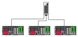
When an error occurs in a normal station, data link can be continued with the stations that are operating normally.
