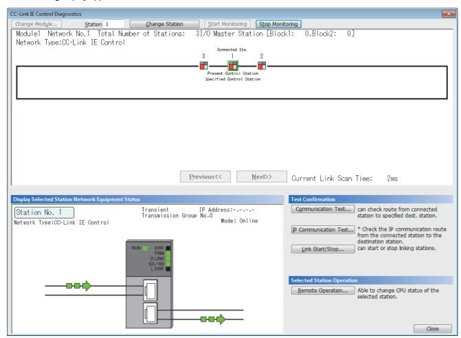
When an icon indicating an error is displayed in "Network information display" in the "CC-Link IE Control Diagnostics", use the CC-Link IE Controller Network diagnostics to identify the cause of the error and take actions. ( MELSEC iQ-R CC-Link IE Controller Network User's Manual (Application))
