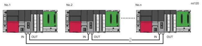
The RJ71GP21(S)-SX has IN connector and OUT connector. Connect the IN connector of own station to OUT connector of another station and OUT connector of own station to IN connector of another station.
