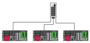
When an error occurs in a device station, data link can be continued with the stations that are operating normally.
