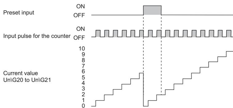
The preset is executed when the preset input changes OFF→ON.
