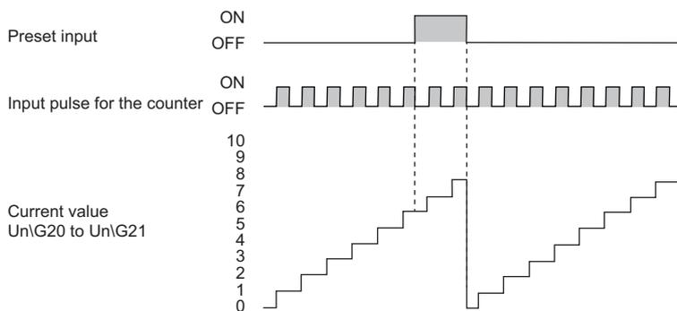
The preset is executed when the preset input changes ON→OFF.
