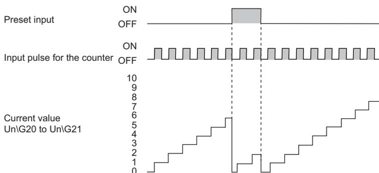
The preset is executed when the preset input changes OFF→ON and when it changes ON→OFF.
