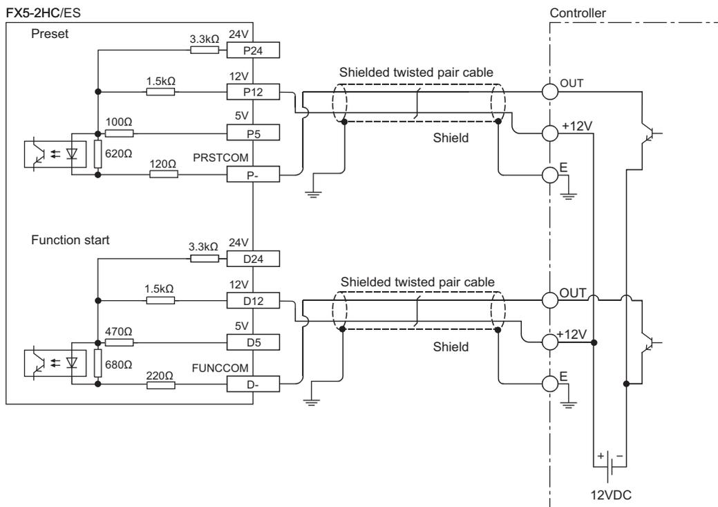
■When the controller (sink load type) has a voltage of 5VDC
