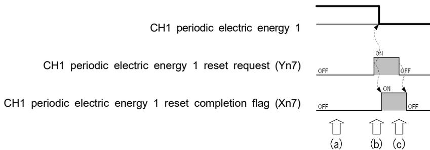
Figure 4.2.2-2 How to reset the periodic electric energy
