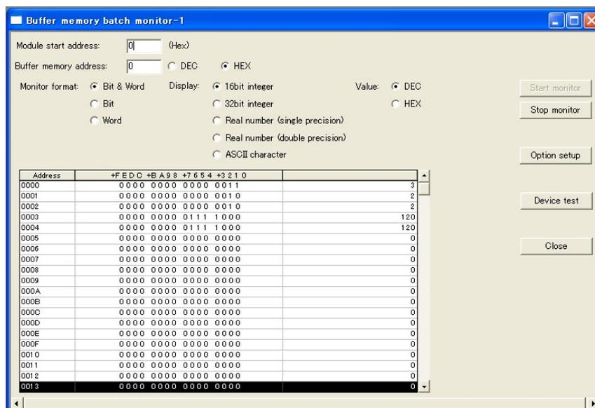
Figure 8.7.3-1 Dialog box to monitor all buffer memories (a case where the module is attached to the slot 0)
