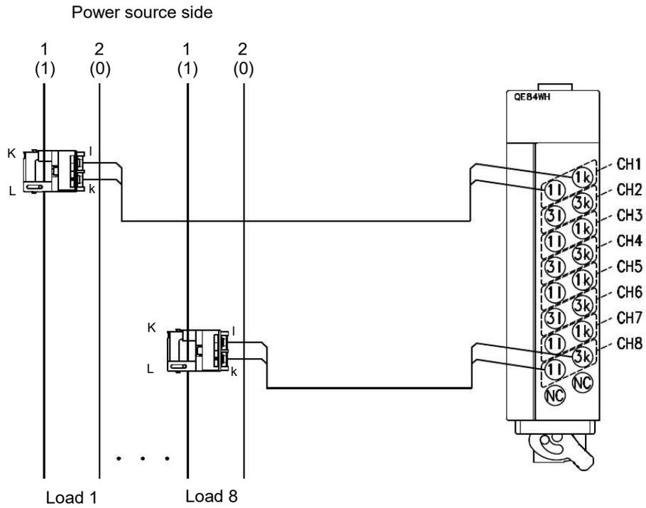
Figure 9.3-2 Example of wiring using a sample program
