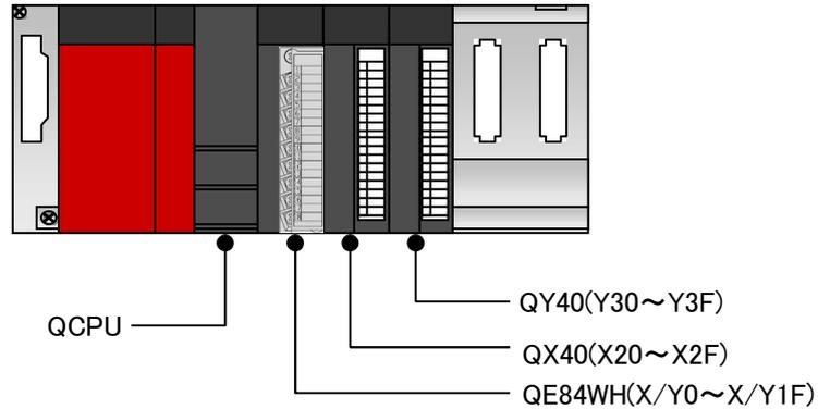
Figure 9.2-1 Sample system configuration using a sample program
