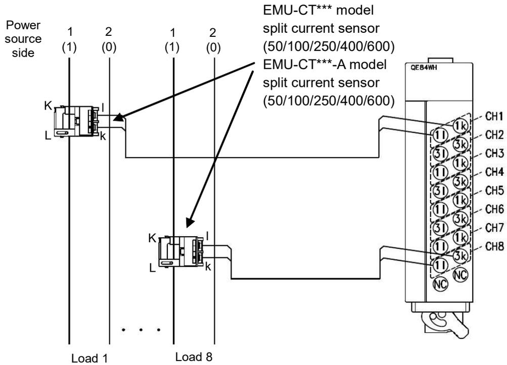
Figure7.7(2) Wiring in the using split current sensor
