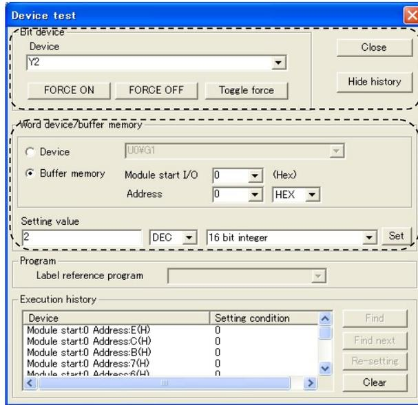
Figure 7.9.3-2 Device test dialog box (a case where this module is attached to the slot 0)
