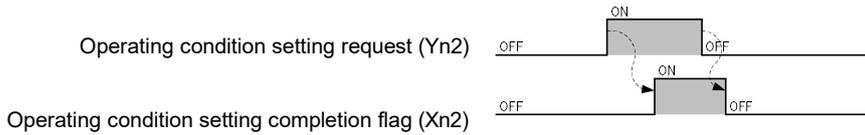
Figure 4.2.4-1 Time chart of alarm monitoring setting
