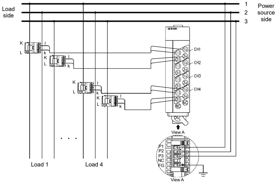
Figure 9.2-2 Example of wiring using a sample program
