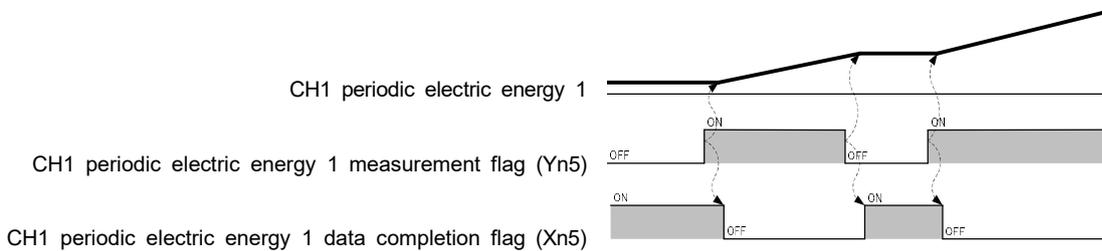
Figure 4.2.2-3 Example of continuous measurement of periodic electric energy
