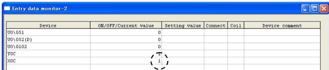
Figure 8.7.4-3 Checking the device “XC”<sup>\*</sup> in the dialog box to Entry data monitor
