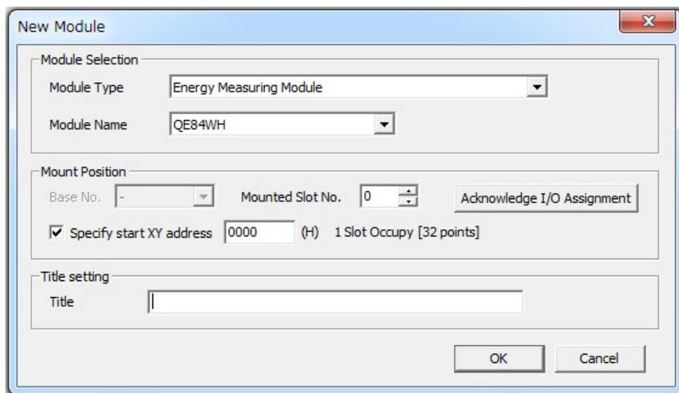
Figure 8.6.1-1 Dialog box of “I/O assignment”
