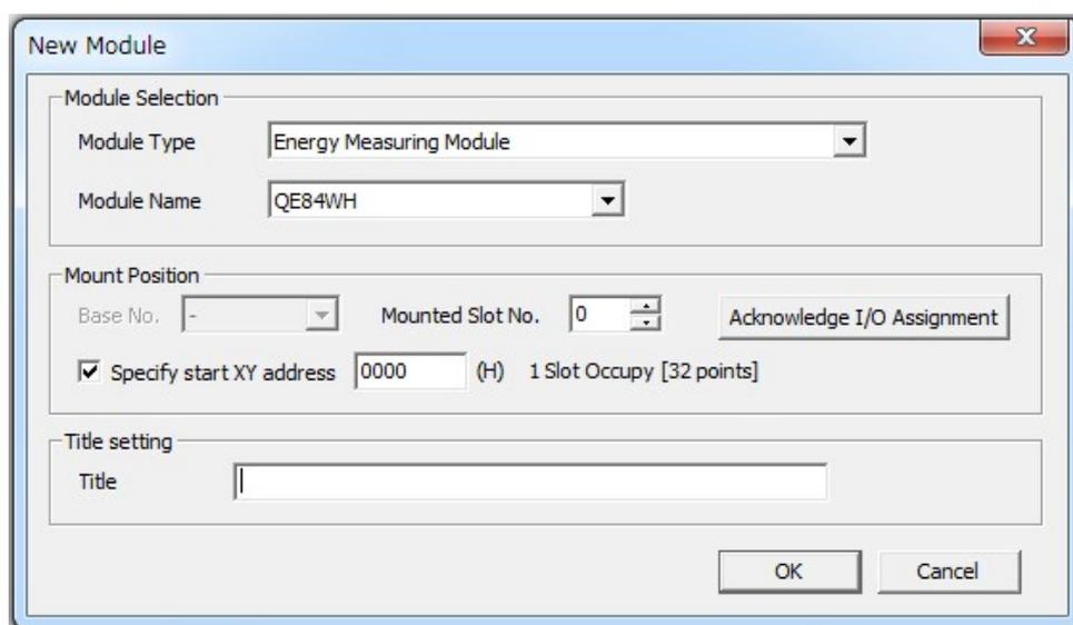
Figure 7.8.1-1 Dialog box of “I/O assignment”
