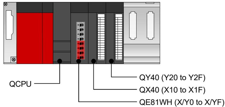
Figure 8.2-1 Sample system configuration using a sample program
