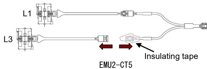
■ Extending the cable of 5 A current sensor
