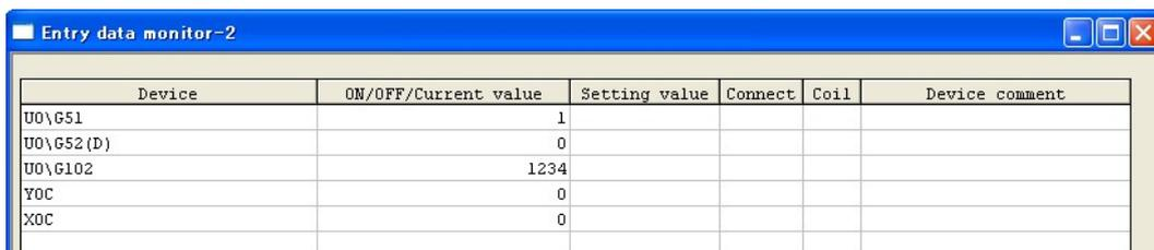
Figure 7.7.4-1 Dialog box to Entry data monitor (a case where the module is attached to the slot 0)
