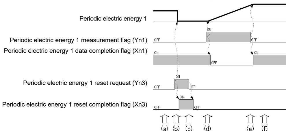
Figure 4.2.2-4 Example of measurement of periodic electric energy after every reset
