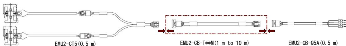
◆ Connecting 5 A current sensor and extension cable (separate)
