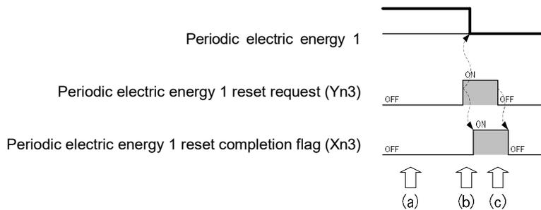
Figure 4.2.2-2 How to reset the periodic electric energy
