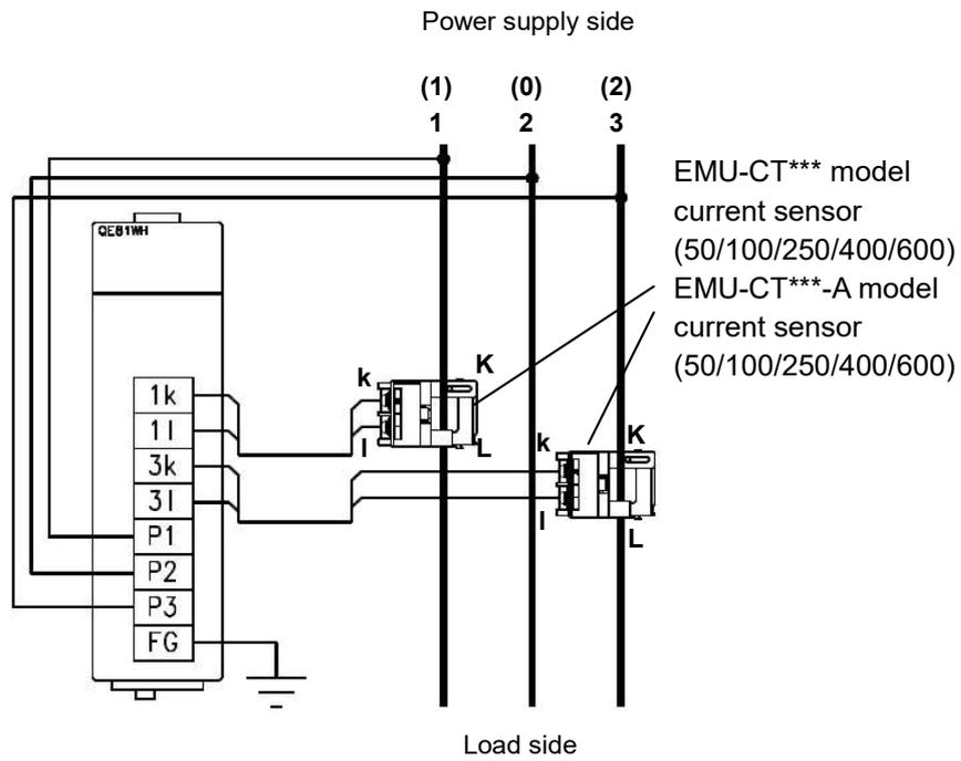
Figure 7.5.3(2)-(c) In the case of Single-phase 3-wire
