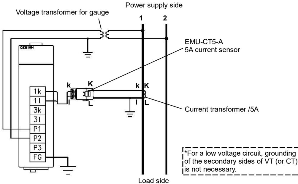
Figure 7.5.3(1)-(b) In the case of Single-phase 2-wire system (with the voltage transformer for gauge/current transformer)
