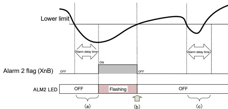
Figure 4.2.4-4 Time chart of the upper/lower limit alarm (alarm reset method = “auto-reset”)
