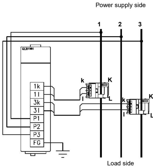
Figure 8.2-2 Example of wiring using a sample program
