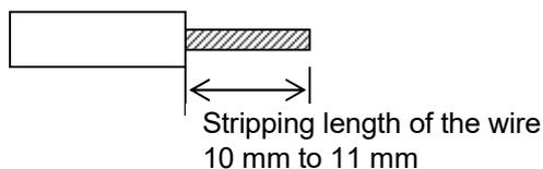
(4) When stranded wire is used, a bar terminal must be used.
