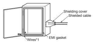
\*1. These wires are used to improve the conductivity between the door and control cabinet.
