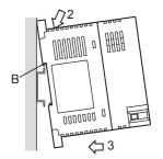
4 Lock the DIN rail mounting hooks (A in the following figure) while pressing the PLC against the DIN rail.
