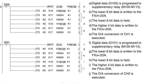
Digital to analog conversion execution input of CH1 :X000 Digital to analog conversion execution input of CH2 :X001
