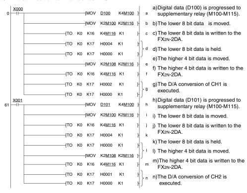
Digital to analog conversion execution input of CH1 :X000 Digital to analog conversion execution input of CH2 :X001
