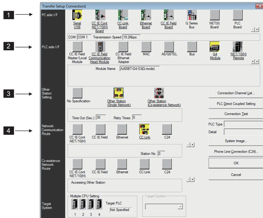
Figure 6.14 [Transfer Setup] dialog box
