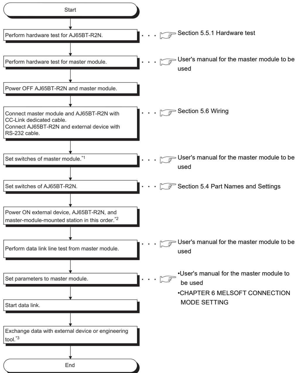
**Figure 5.1 Preparatory procedures and setting**
