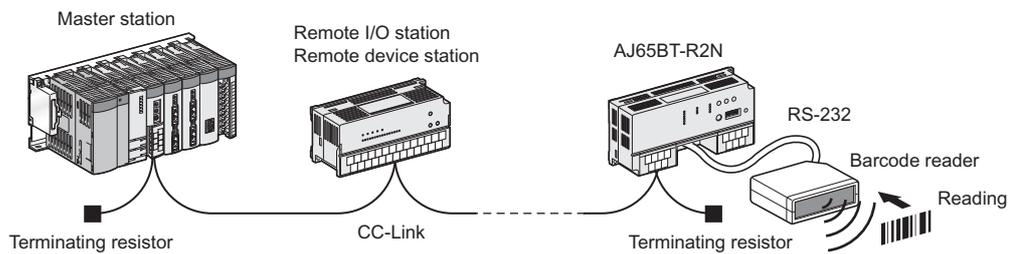
Figure 2.1 When connecting a barcode reader
