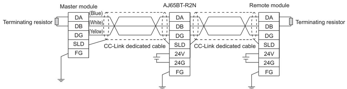
Figure 5.8 Connection between AJ65BT-R2N and master module
