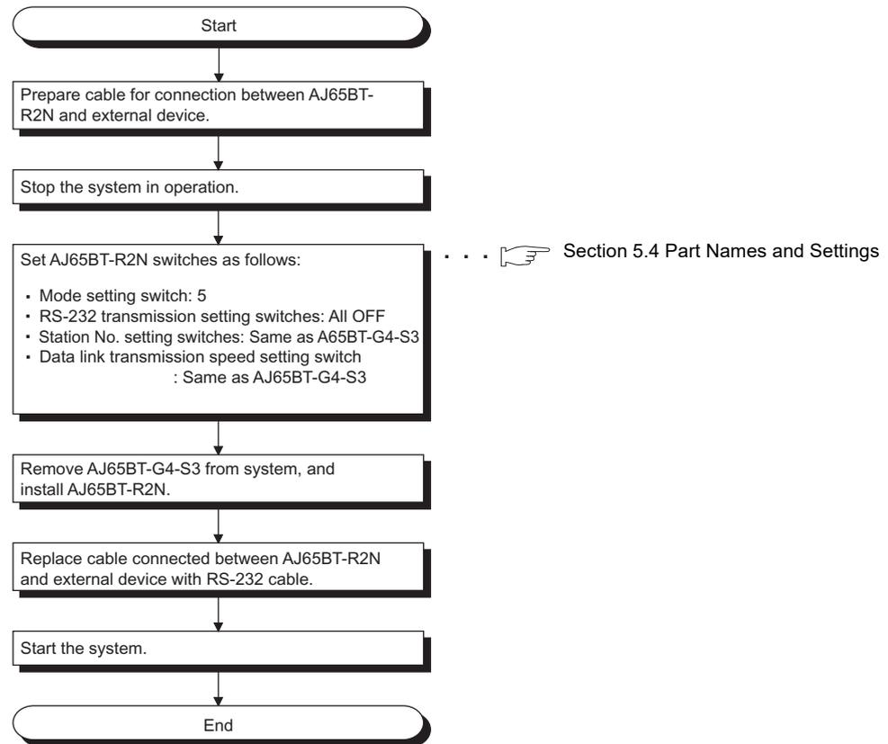
Figure App.1 Procedures for replacing AJ65BT-G4-S3 with AJ65BT-R2N
