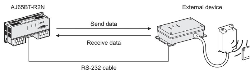
Figure 1.3 Nonprocedural communication function
