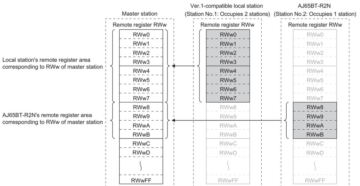
Figure 3.3 Example of remote register area
