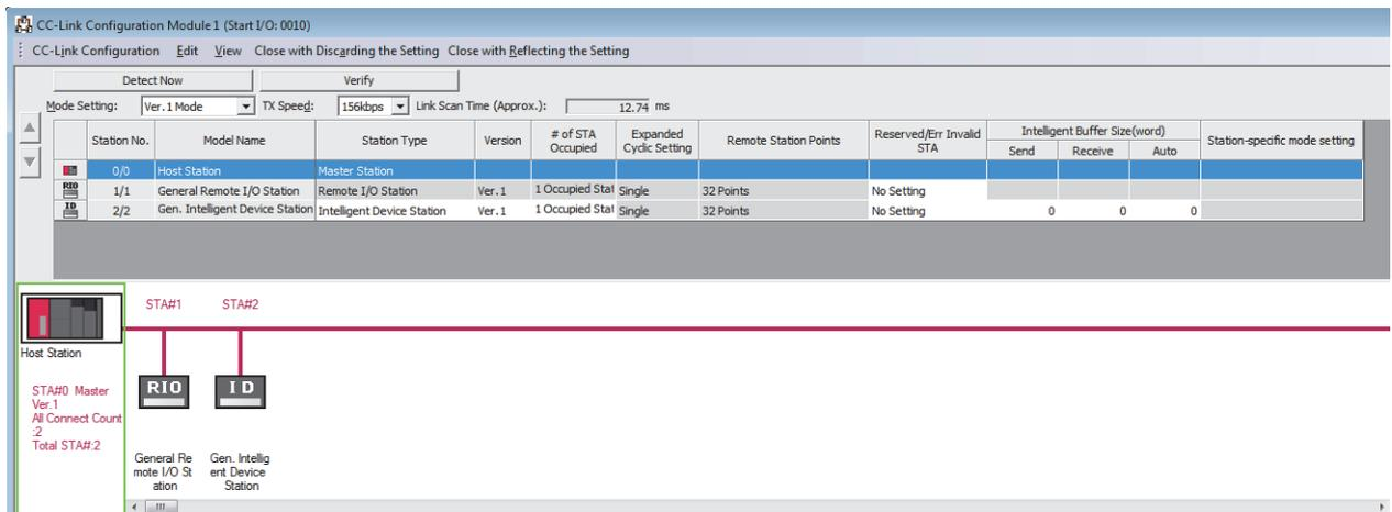
Figure 6.5 [CC-Link Configuration Module 1] dialog box
