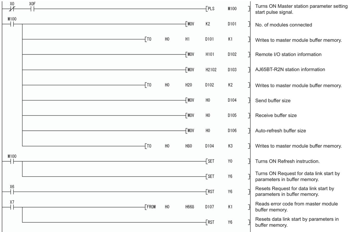
Figure 6.17 Program example when using FROM/TO instruction
