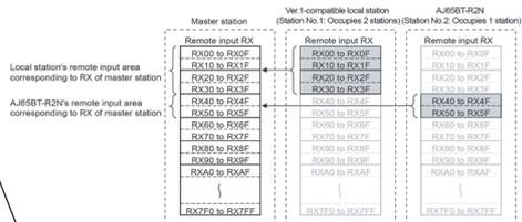
Figure 3.2 Example of remote input area
