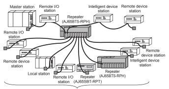
Star-topology wiring with 8 branch lines can be used!!
