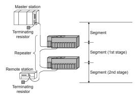
(4) Instructions for using different models of repeaters in combination Note that when combining the repeaters of different models, there are the following restrictions on the number of connectable repeaters and the number of connected stages.
