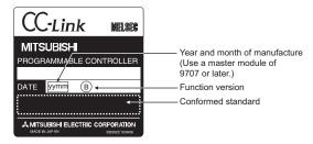
(b) Rating plate of A1SJ61BT11 or A1SJ61QBT11
