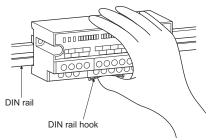
(5) When installing the AJ65SBT-RPT module on the control panel, to improve the ventilation and facilitate the replacement of the module, provide a distance of 60 mm (2.36inch) or longer between the upper and lower surfaces of the module and the structural members or parts.
