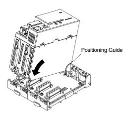
3) Tighten the base fixing screw with a screw driver (stem length: 70 mm/2.76" or more) (torque 0.5  $N{\cdot}m)$
