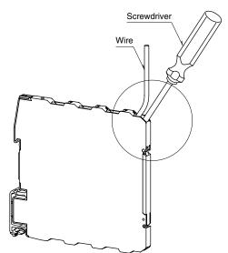
1) Insert a minus screwdriver into the wire entry opening, between the clamp and the housing, until its tip hits the bottom where it is firmly held.
