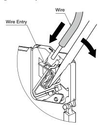
3) Confirm that the wire tip hits the bottom and pull out the screwdriver in holding it in position.
