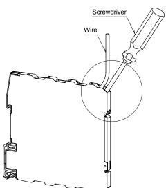
1) Insert a minus screwdriver into the wire entry opening, between the clamp and the housing, until its tip hits the bottom where it is firmly held.
