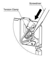
Insert a wire. Push the screwdriver toward the direction indicated with the arrow in the figure below to widen the opening if necessary.
