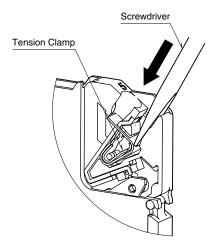
2) Insert a wire. Push the screwdriver toward the direction indicated with the arrow in the figure below to widen the opening if necessary.
