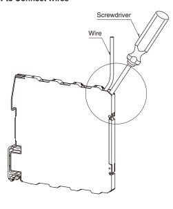
1) Insert a minus screwdriver into the wire entry opening, between the clamp and the housing, until its tip hits the bottom where it is firmly held.
