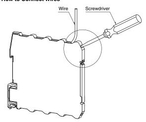
Insert a wire. Confirm that the wire tip hits the bottom and tighten the screw with a screwdriver.
