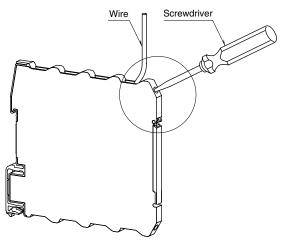
Insert a wire. Confirm that the wire tip hits the bottom and tighten the screw with a screwdriver.
