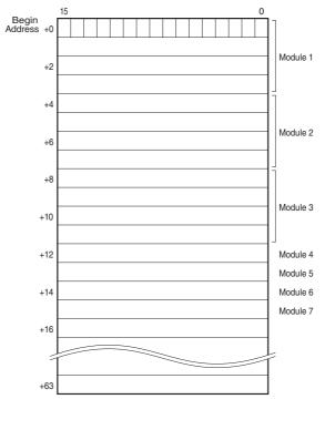
Module Status, Error Status and Data Error Status are assigned to +64, +65 and +66 respectively. Each module can handle either input or output data. Input and output cannot be mixed in one module. Input data from the master device is transferred to the module's output data area. The master device can read from the output data area the data it has set.
