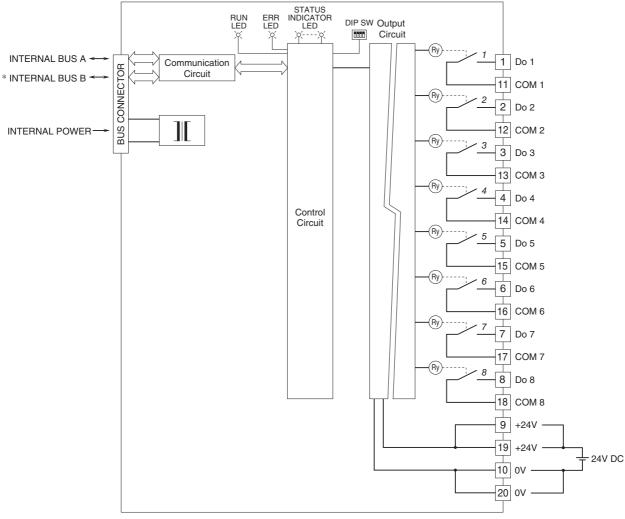
Numbers in italic indicate LED No.s assigned to the front panel LEDs.
