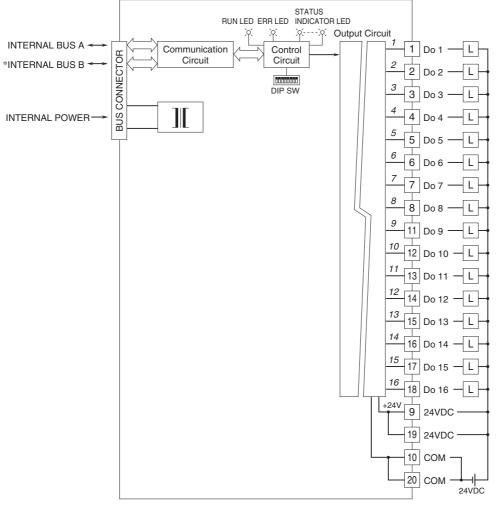
Numbers in italic indicate LED No.s assigned to the front panel LEDs. \*For dual redundant communication. Specifications are subject to change without notice.
