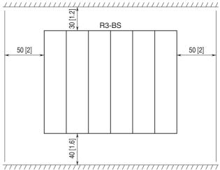
Panel bottom or wiring conduit (height ≤ 50 mm or 2 in.)
