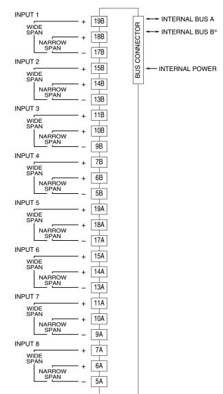
**Wide span:** -10 - +10 V DC, -5 - +5 V DC, 0 - 10 V DC, 0 - 5 V DC, 1 - 5 V DC
