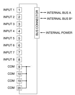
\*For dual redundant communication. Note: Do not use viod terminals
