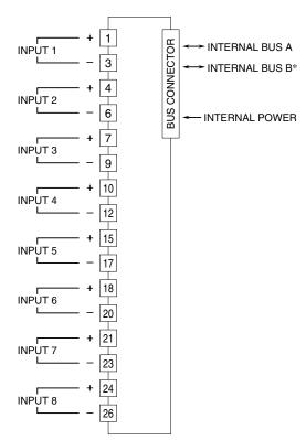
\*For dual redundant communication. DO NOT connect external wiring to the unused terminals.
