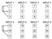
Unused channels left open are equal to the burnout, which turns the red ERR LED on and sets a burnout flag at the PLC or the host device.
