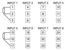
The resistance value must match the RTD type (100 $\Omega$  for Pt 100, 50 $\Omega$  for Pt 50 $\Omega$ ).
