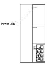
**Power LED**: Green LED turns on when the power is supplied.
