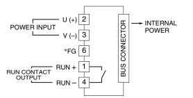
\*In order to improve EMC performance, bond the FG terminal to the ground. Caution: This terminal is NOT a protective conductor terminal.
