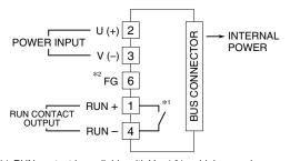
\*1. RUN contact is available with Ver.1.01 or higher versions.\*2. In order to improve EMC performance, bond the FG terminal to the ground.
