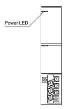
**Power LED**: Green LED turns on when the power is supplied.
