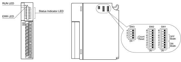
Count Reset SW must be turned off during operation.
