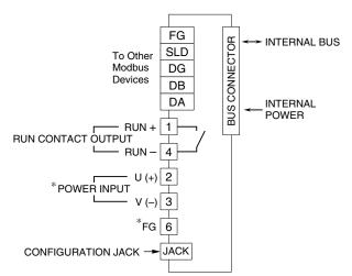
\*Not provided with 'No Power Supply' type module. Caution: FG terminal is NOT a protective conductor terminal.
