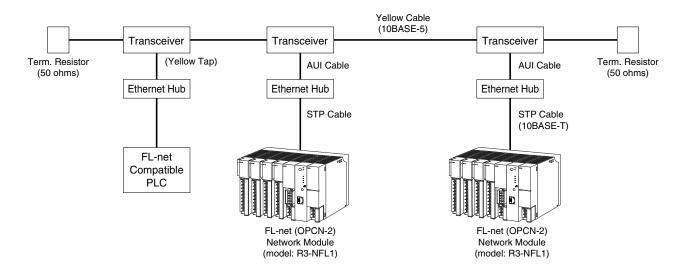
A small system can be configured only with Ethernet hubs. Multiple hubs can be interconnected via twisted-pair cables to expand it, and fiber optics media converters are used to connect to those in remote locations. Choose appropriate types of hubs which can be connected via 10BASE5 or 10BASE2 cables if they are to be used with the FL-net.
