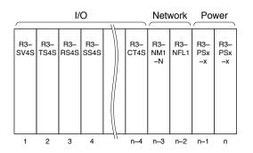
The builder software identifies each I/O module by its I/O address, normally its slot (position) number assigned from the left (I/O 1) to the right (I/O n) on the R3-BSx base. The positions may be freely arranged with the R3-BSWx base which is provided with address setting switches for each slot.
