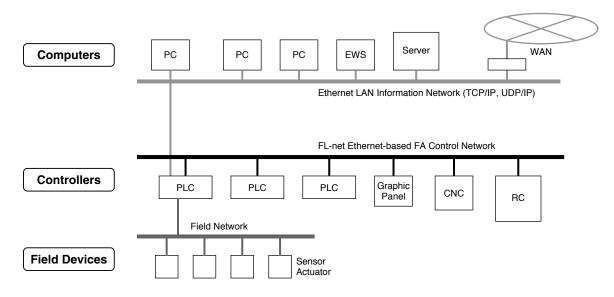
FL-net (OPCN-2), which has been established in the JIS (Japan Industrial Standards) and the JEM (Japan Electrical Manufacturers) standards, is adopted by most PLC manufacturers. Detailed information such as the certified products list, FL-net specifications and implementation guides is available at the Open PLC Network (OPCN) in the Japan Electrical Manufacturers Association (JEMA) web site: http://jema-net.or.jp/Japanese/hyojun/opcn-e/top-opcn.htm.
