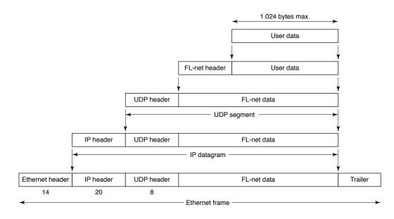
The following diagram shows an example of FL-net data for a single frame that can be observed on the communications line. 128 bytes of cyclic data is being transferred.
