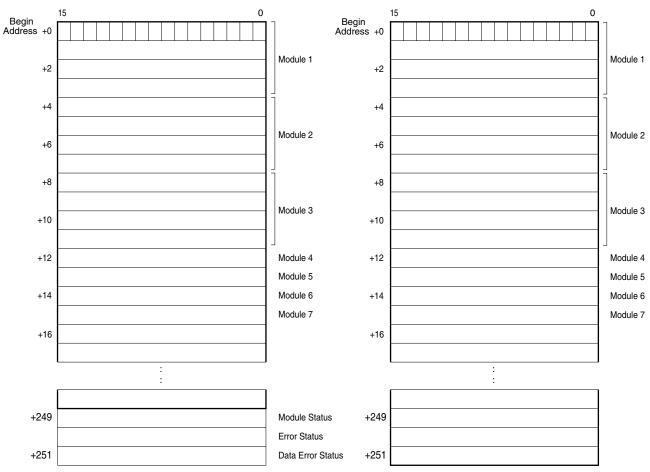
The area enclosed with bold line is assigned for I/O data
