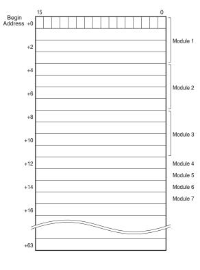
Module Status, Error Status and Data Error Status are assigned to +64, +65 and +66 respectively.
