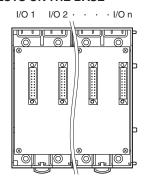
With Model R3-BS base, mount the I/O Modules from the left end (I/O 1) to the right in order that the Network Module assigns data areas from I/O 1.
