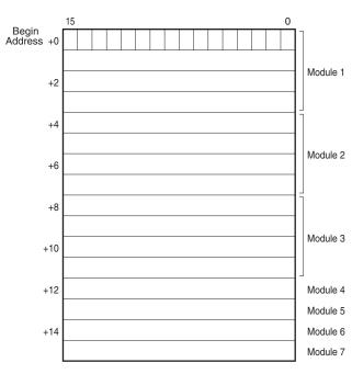
Module Status, Error Status and Data Error Status are assigned to +16, +17 and +18 respectively. Each module can handle either input or output data. Input and output cannot be mixed in one module. Input data from the master device is transferred to the module's output data area. The master device can read from the output data area the data it has set.
