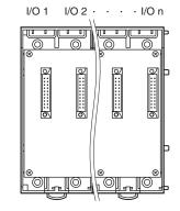
With Model R3-BS base, mount the I/O Modules from the left end (I/O 1) to the right in order that the Network Module assigns data areas from I/O 1.
