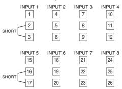
The input will become unstable if unused channels are left open. Unused channels can be specified and set so on the PC Configurator Software (model: R3CON) without needing to short at the field terminals.
