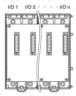
With Model R3-BS base, mount the I/O Modules from the left end (I/O 1) to the right in order that the Network Module assigns data areas from I/O 1.
