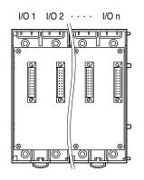
When using R3-BS, mount the modules starting from I/O1 (the interface modules are assigned from I/O1).
