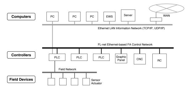
FL-net (OPCN-2), which has been established in the JIS (Japan Industrial Standards) and the JEM (Japan Electrical Manufacturers) standards, is adopted by most PLC manufacturers. Detailed information such as the certified products list, FL-net specifications and implementation guides is available at the Open PLC Network (OPCN) in the Japan Electrical Manufacturers Association (JEMA) web site: http://www.jema-net.or.jp/Japanese/hyojun/opcn/index.htm.
