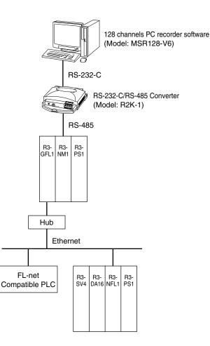
R3-GFL1 can be used as a gateway for different protocols by combination of R3-Nx. A small system can be configured only with Ethernet hubs. Multiple hubs can be interconnected via twisted-pair cables to expand it, and fiber optics media converters are used to connect to those in remote locations. Choose appropriate types of hubs which can be connected via 10BASE5 or 10BASE2 cables if they are to be used with the FL-net.
