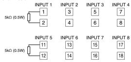
Unused channels left open are equal to the input lower than -15%, which sets a data abnormality at the PLC or the host device.
