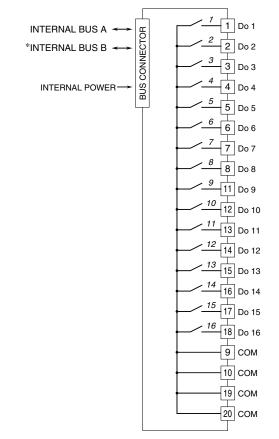
Numbers in italic indicate LED No.s assigned to the front panel LEDs. \* For dual redundant communication.
