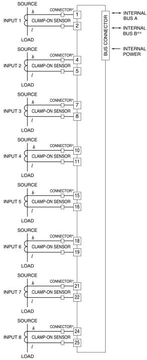
\* Connector provided only for the CLSA-08 and CLSA-12. \*\* For dual redundant communication.
