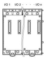
Mount the I/O Modules from the left end (I/O 1) to the right in order that the Network Module assigns data areas from I/O 1.
