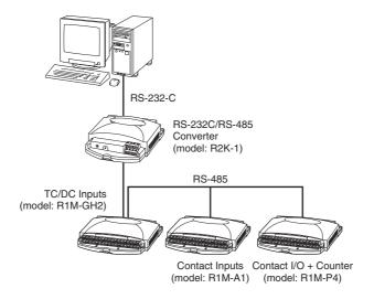
When the cable distance between the PC and the R1Ms is long, insert an RS-232-C/RS-485 Converter for isolation.
