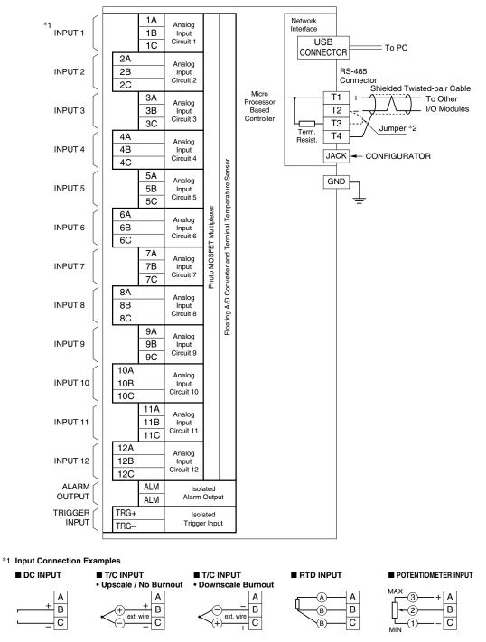
\*2 When the device is located at the end of a transmission line via twisted-pair cable, (when there is no cross-wiring), close across the terminal T2 – T3 with the attached jumper pin (or with a leadwire). When the device is not at the end, remove the jumper pin.
